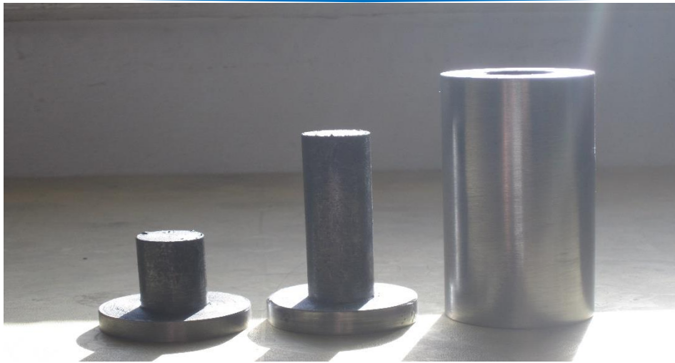
Fig. 1 Compressibility die of coarse particles.
